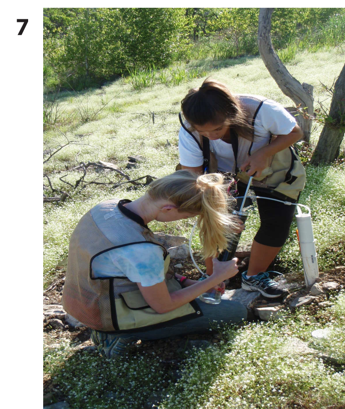
Figure 7 shows the process of removing water from the lysimeters using a vacuum flask and pump.
