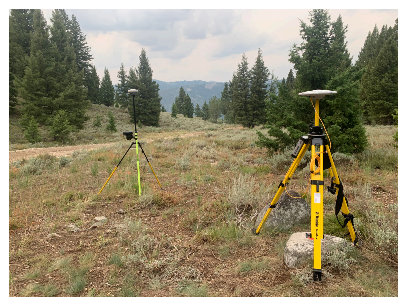
Figure 3. Trimble GPS base station (right) and mobile receiver.
