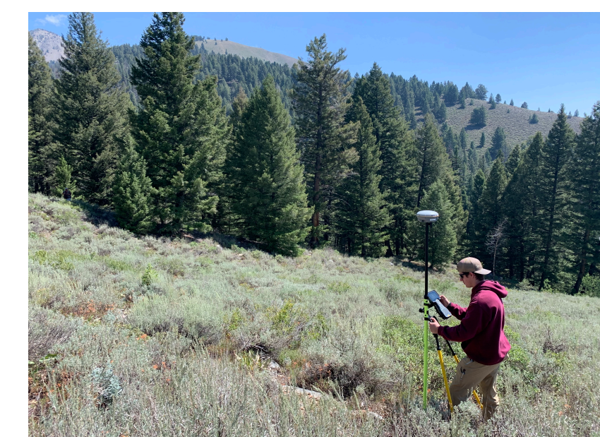
Figure 6. Field assistant using the Trimble mobile receiver to collect positions on Profile 5.
