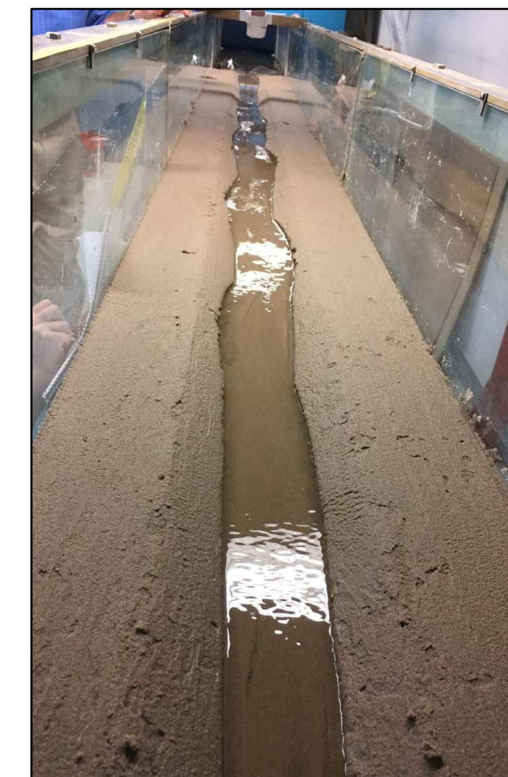
Figures 10 and 11: Channel that developed natural meanders with an adverse pressure gradient (slope change) downstream.
