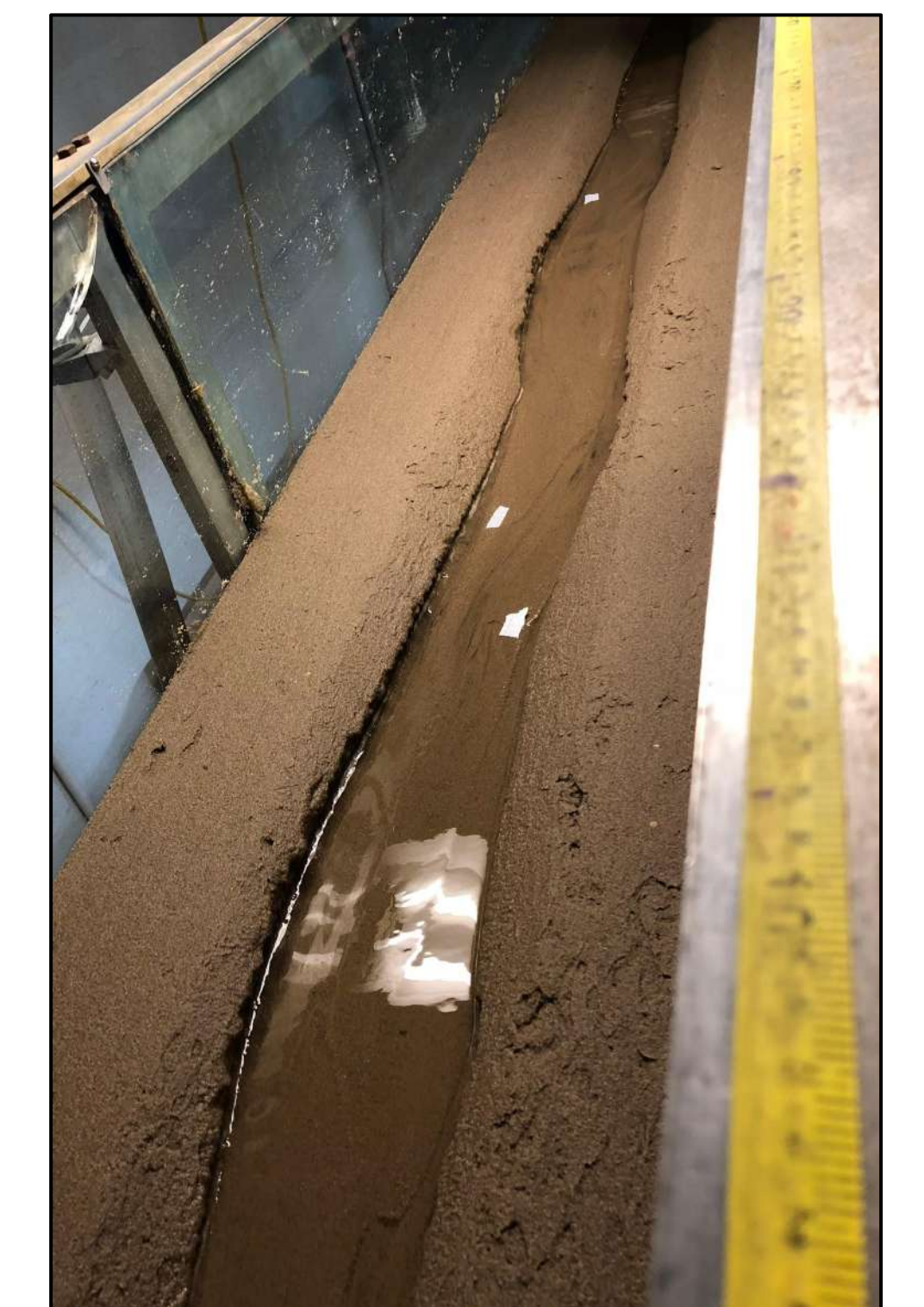
Figures 10 and 11: Channel that developed natural meanders with an adverse pressure gradient (slope change) downstream.
