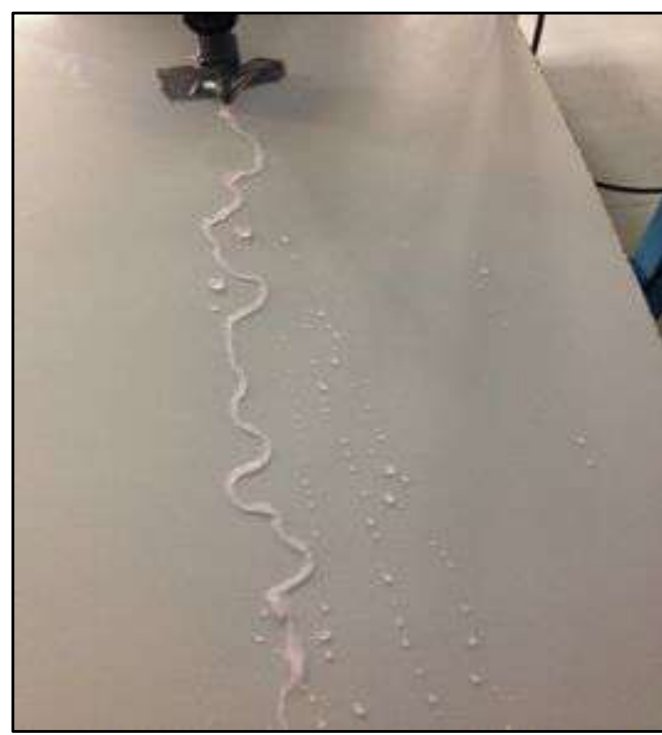
Figure 4: Meanders in rivulets generated on inclined surfaces with a steady laminar stream of water under adjustable hydraulic head.
