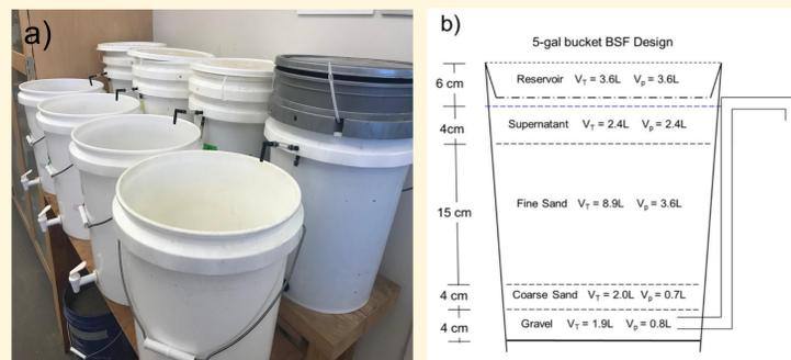
Figure 2. (a) photograph of the BSF setup. (b) 5 gallon bucket design created in collaboration with CAWST.
