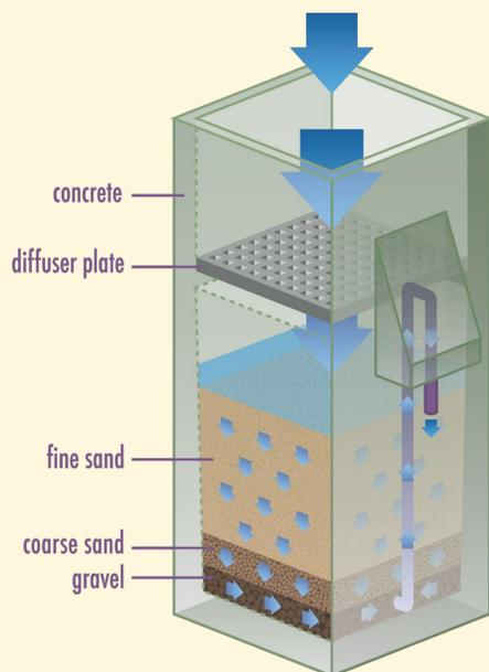
Using concrete and sand, these biosand water filters remove impurities and provide water for drinking and cooking.
