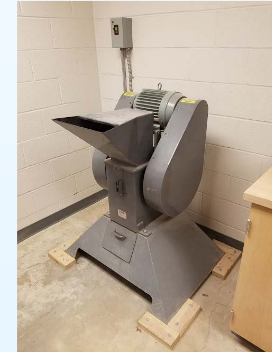
Crush river sand and aggregates until material can pass through number 20 sieve
