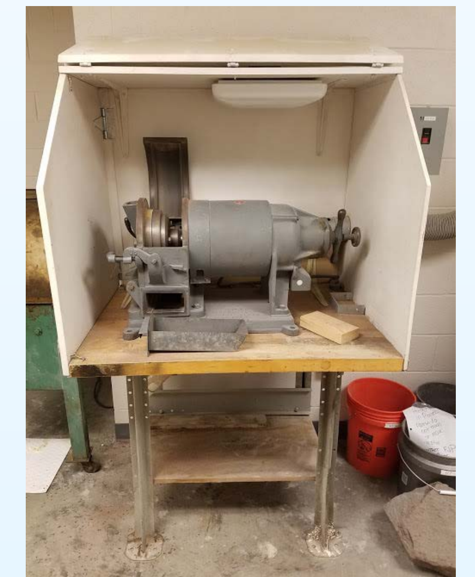
Crush river sand and aggregates until material can pass through number 20 sieve
