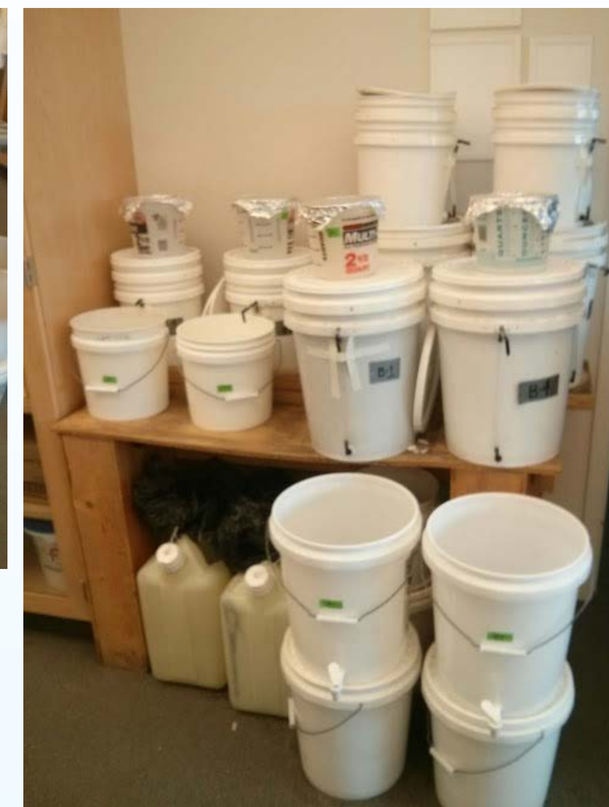
Two 5-gallon bucket BSFs -1 untreated river sand -1 disinfected river sand
