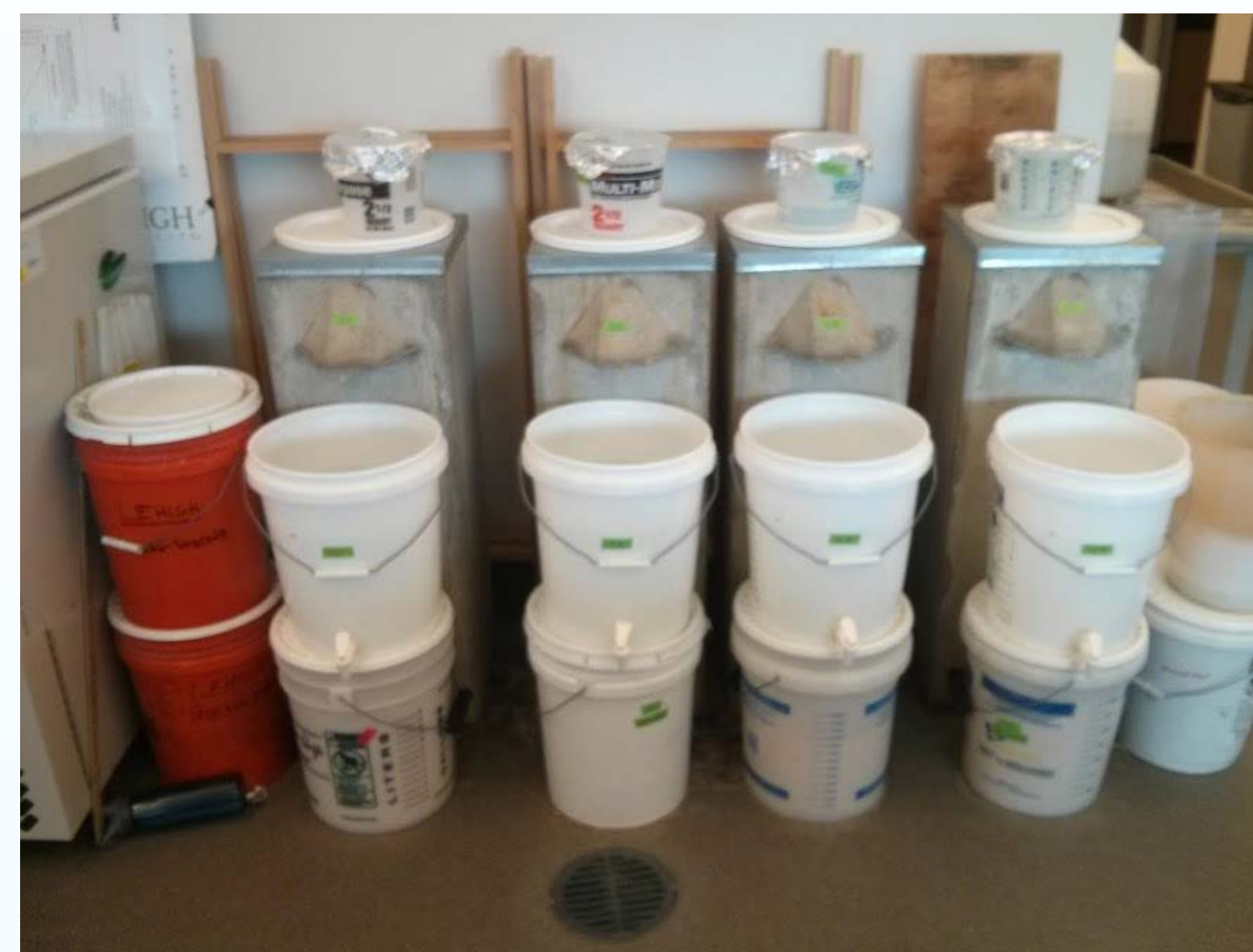
Four full-scale concrete BSFs - 2 control - 1 untreated river sand - 1 disinfected river sand
