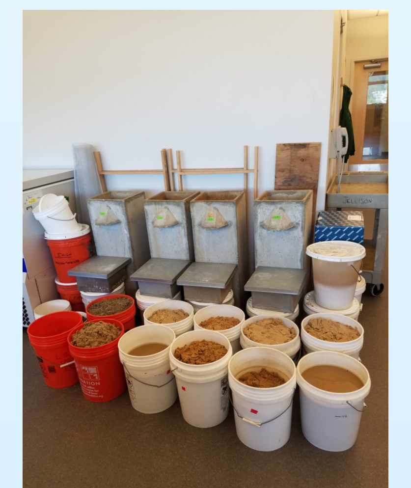
Crush river sand and aggregates until material can pass through number 20 sieve
